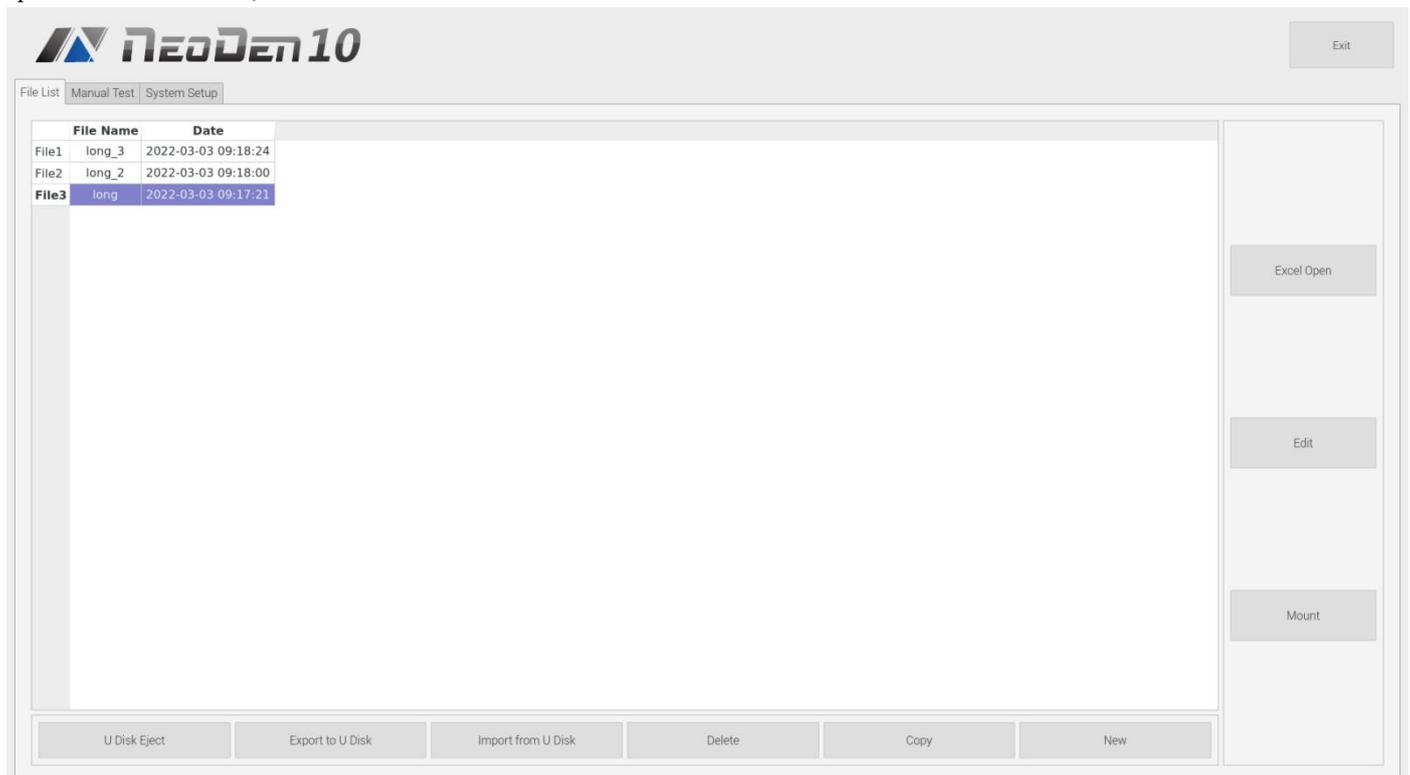
When want to do mount of the finished working file,need choose the phase 1 file(e.g. long),then click mount.(the long tracks also support mount 2 phases,then only need create 2 working files).
