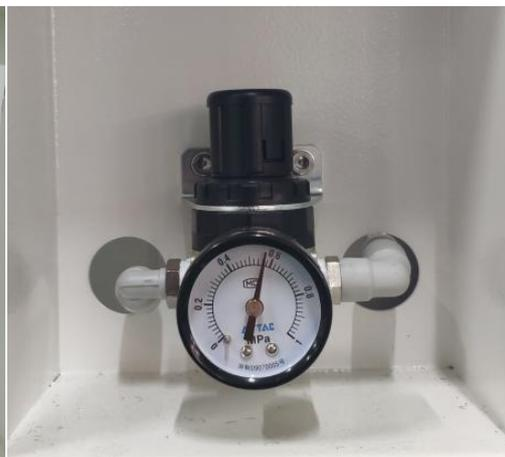
figure 7-feeder pressure 0.55MP
