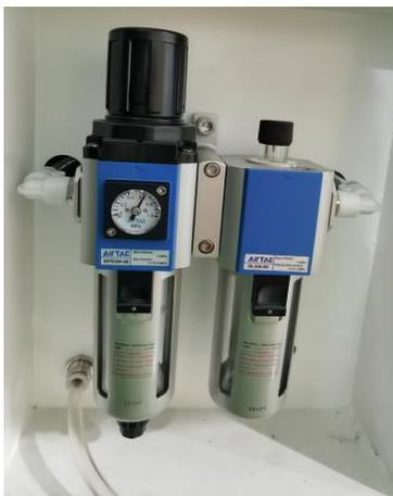
figure 6- oil-water separator
