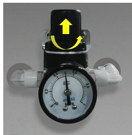
Figure 7- Feeder Pressure 0.5MP
