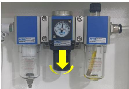
Figure 6-The air supply of the equipment shall not be less than 0.55MP
