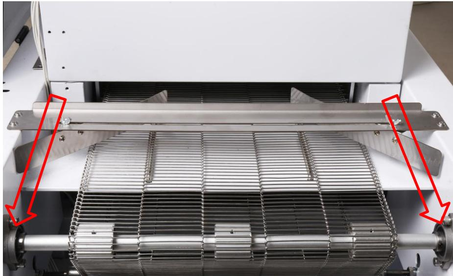
◆Regularly add high temperature lubricating oil to transfer chain bearings.
