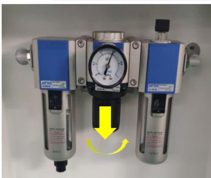
Figure 6-The air supply of the equipment shall not be less than 0.6MP
