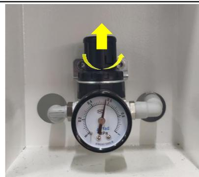
Figure 7- Feeder Pressure 0.55MP
